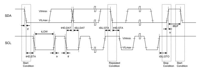
Figure 8.2 2-wire serial interface timing definition
