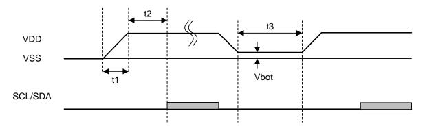
Figure 8.1 V<sub>DD</sub> supply timing
